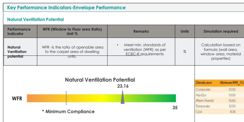
Figure 17 : Envelope Performance indicator - Window to Floor Area Ratio.
