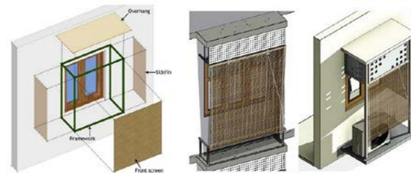
**Figure 4 : Protection through shading**
