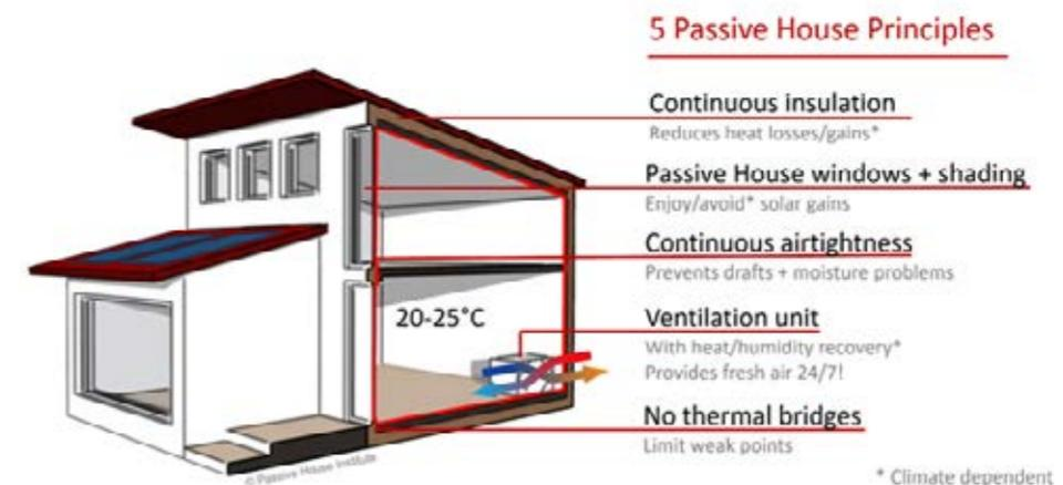
**Figure 25 :** The five Passive House Principles. [Source PHI]
