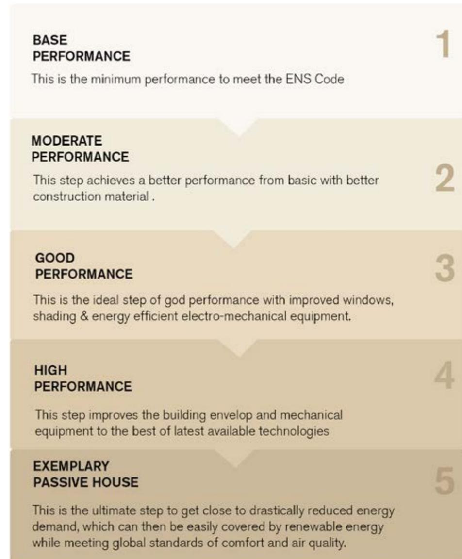
Figure 7 : The step-by-step energy performance improvement
