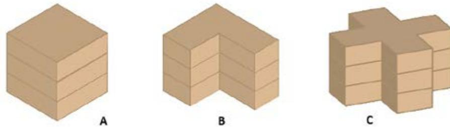
**Figure 3 : Compactness of Building** - Compactness depends on the geometry of the building and it varies with the building typology. In this figure the surface to volume ratio increases from A to C as the built form gets more complicated, the compactness reduces.
