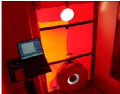
Figure 28 : Airtightness test [Source PHI]
